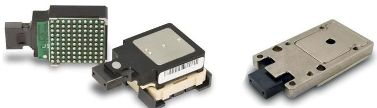
These transceivers can be soldered or socketed to a printed circuit board and are well suited for small, compact systems requiring high I/O density, low power, and small space. Many of these transceivers have been qualified to operate in harsh environments, such as the ones found in space, and aerospace and defense applications.
