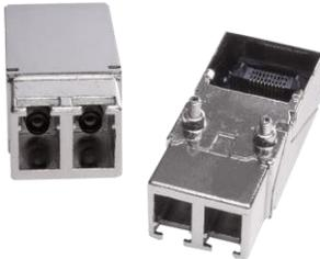
Moog Stiletto series optical fiber transceivers consist of 10 Gbps optoelectronic transmitter and receiver functions integrated into a pluggable Duplex LC compliant connector. The optical harsh environment transmitters are 850 nm VCSEL lasers. The transmitter input lines are driven with differential CML signals applied to the transmitter (TX+ and TX-) lines. Dual loop, temperature compensated, VCSEL drivers convert the transmitter input signals to suitable VCSEL bias and modulation currents.
